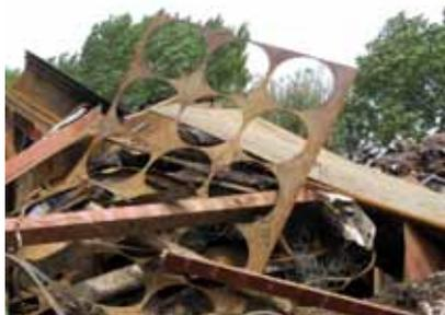
A typical 'skeleton', left over after blanking
